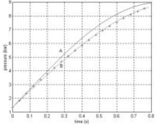
**Fig. 1** Pressure changes during the filling of a chamber, '+' experimental results, computer simulation with the use of (A) ISO 6358 and (B) Saint Venant-Wantzel with changeable  $\mu$
